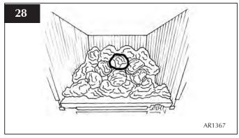
9.11 Place two small coals to the left and right-hand side of the bed in the two spaces left. See Diagram 29.
